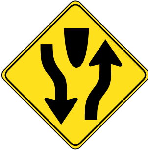
Two-lane highway ends; divided highway begins.
