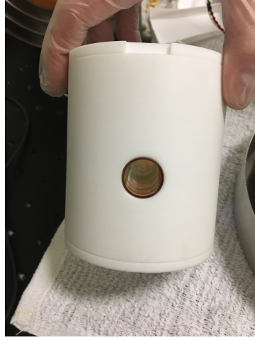
(b) The resistive Teflon oven (TwinLeaf LLC) containing the vapor cell.
