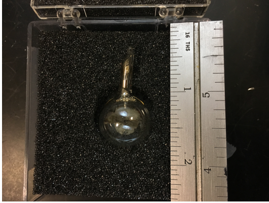
(a) The vapor cell used in the experiment. It is spherical, with an inner diameter is about 1 cm.
