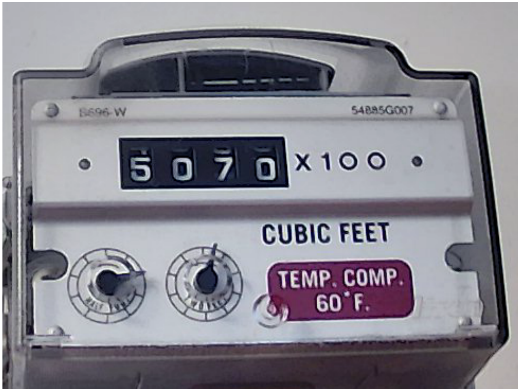
Figure 1.1: Image of the gasmeter taken with a USB webcam and a python script.
