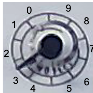
Figure 4.10: The goal of the software is to classify the dials depending on the location of the needle. Assuming that each increment of 0.05 represents a category, the dials will have 10 different regions that will determine the value of the needle.
