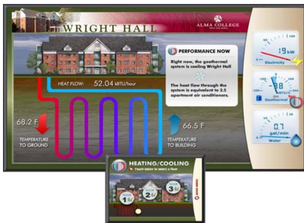
Figure 7. Lobby display and touch screen (inset) displaying geothermal heating system in Wright Hall, a residence hall at Alma College. Color of water in loop and rate of pulsing in loop change in response to monitored conditions to foster a more intuitive
