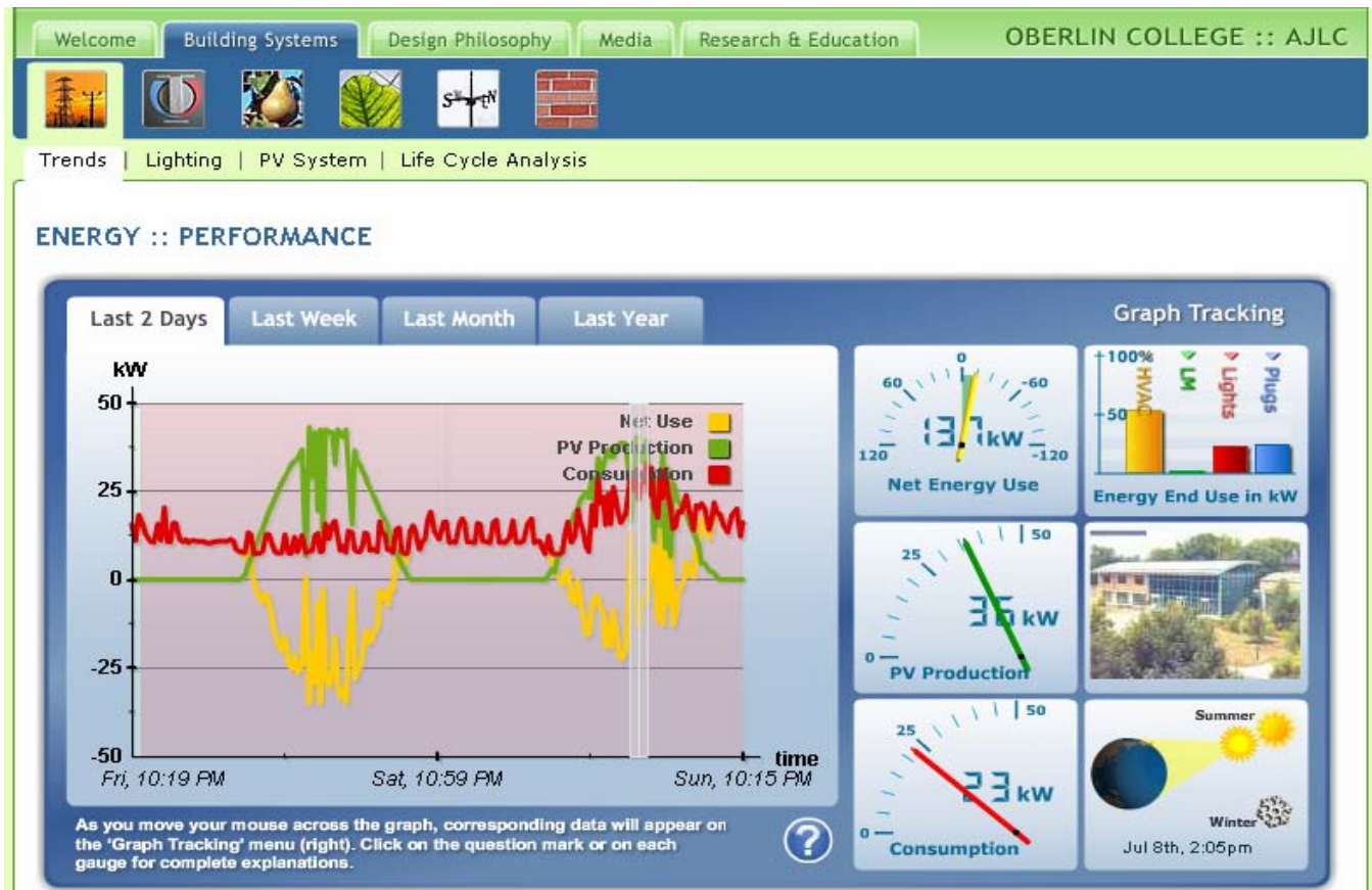
Figure 2. Webpage featuring time series graph of photovoltaic production (green) energy consumption (red) and net consumption (yellow) at the AJLC over a two-day period. On the right, gauges and time lapse photography track performance at any given moment as the data “play” through the time series or as the visitor pulls a control bar back and forth through the time series data. The top right gauge depicts the percentage of electricity at any given moment being consumed through different end-uses (HVAC, Living Machine, lighting and plug loads). The gauge on the bottom right shows changes in the earth’s position relative to the sun (the earth spins as days go by and the angle of the sun changes with the season). Tabs above the graph allow the visitor to display data over a range of time scales. Other portions of the website feature similar real-time data displays for other components of the building and landscape systems.
