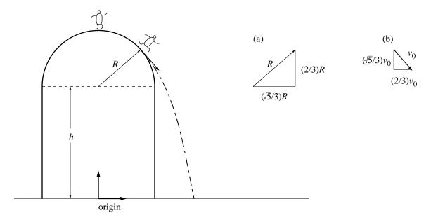
Stage I: Rolling down the dome. The astronomer leaves the dome 1/3 of the way down. The triangle at subfigure (a) shows that this is (2/3)R above the base of the dome, and  $(\sqrt{5}/3)R$  to the right of the center of the dome. (Pythagorean theorem.) That is, he begins free flight at
